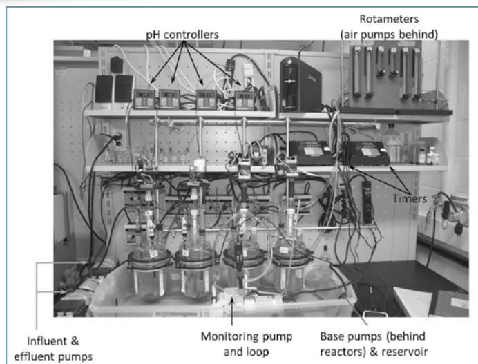
Sequencing batch reactor laboratory setup.
