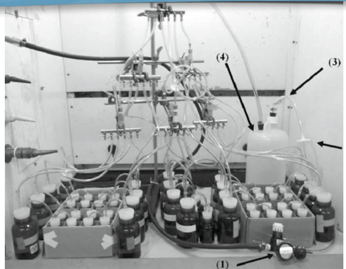
Experimental setup for assessing the biological stability of effluents treated with advanced oxidation process versus those not treated with advanced oxidation process.
