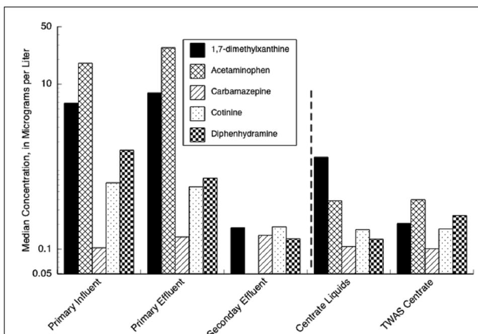
Figure 1. Median Concentrations of Select Pharmaceuticals from Unit Process Samples Common to Plants A-D.
