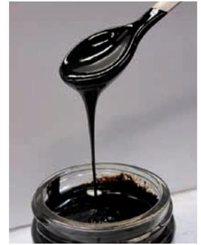
*Biocrude from the HTL test with primary sludge feed.*
