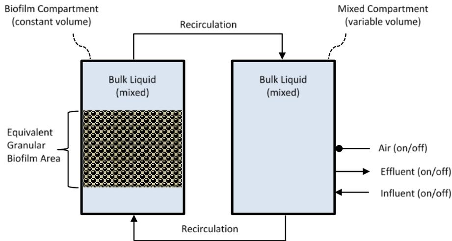
**Schematic of commonly used process configuration in modeling of aerobic granular sludge SBRs.**
