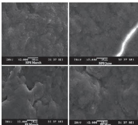
Results of SEM image showing that sludge is a porous surface.
