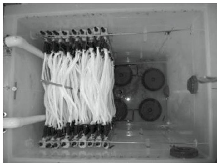
Top down view of membranes in pilot reactor.
