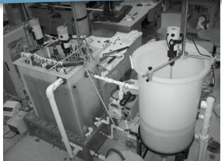
Pilot membrane aerated biofilm reactor at the University of Notre Dame.
