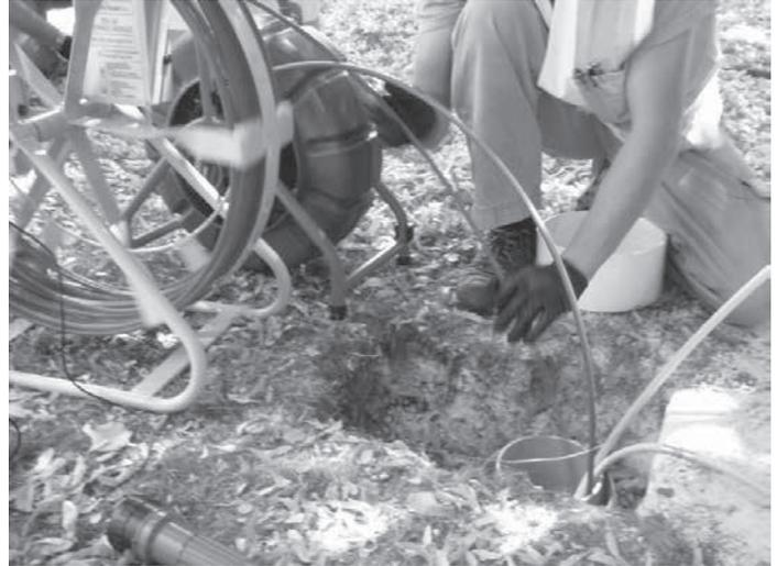
A lateral being tested with Electro Scan.
