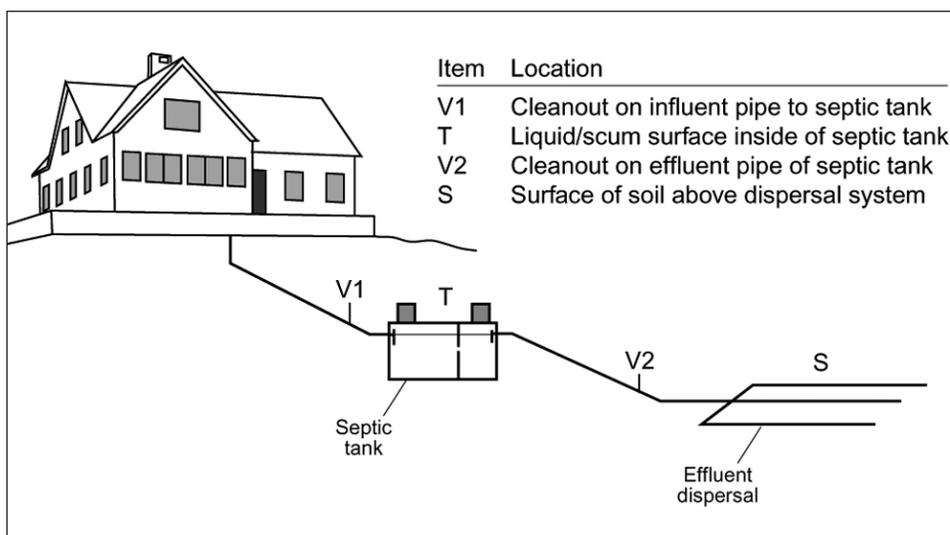
**Definition Sketch for Mass Balance for Total Gas Emission Rate from the Septic System.**
